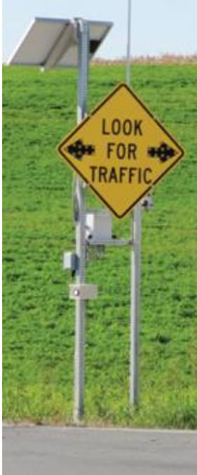
Rural Intersection Conflict Warning System Source: MnDOT Traffic Engineering ( http://www.dot.state.mn.us/trafficeng/signals/conflictwarning.html )
